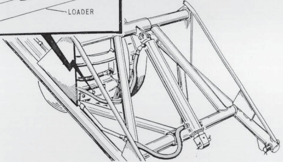
Figure 6 Loader Installation For Ford Models 9N, 2N and Ford-Ferguson Tractors
